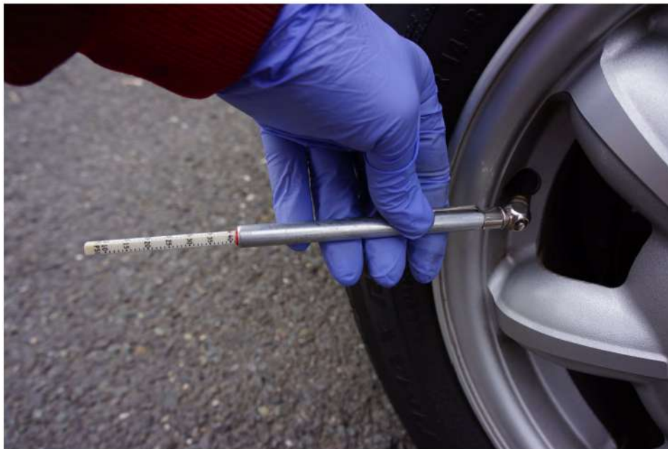
A tire pressure gauge is the least expensive tool you can purchase. Buy one and use it regularly.
